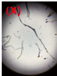
iSperm view of dust/ fiber on the Cover Chip.
